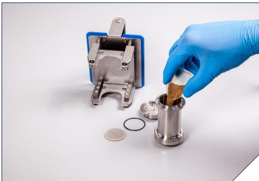
Figure 3 shows the extraction with holder and the unique magnetic lid for the easy closure of the cell
