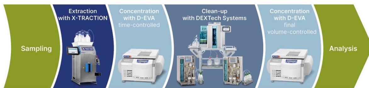
Figure 1. The automated workflow for the extraction, evaporation and clean-up of a variety of POPs (PCBs, PCDD/Fs, PBDEs and PCNs) using LCTech instruments
