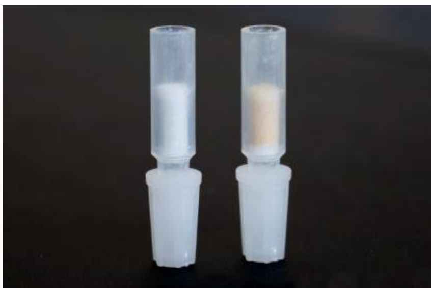
Figure 18: Chili (highly coloured matrix) - left unused CrossTOX® column, right used CrossTOX® column to clean-up the extract
