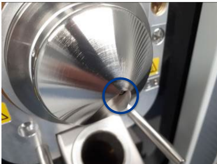
Figure 21: Sweep cone after 150 spice and peanut samples, which were cleaned-up by CrossTOX®.
