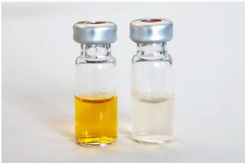
Figure 17: Chili (highly coloured matrix) - left not cleaned crude extract, right purified with CrossTOX® column
