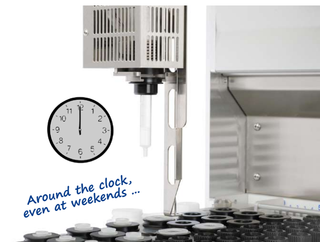
SPE-gripper with immunoaffinity column
