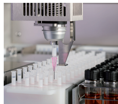
Processing on FREESTYLE ThermELUTE™: Gripper with adapter takes the SMART column
