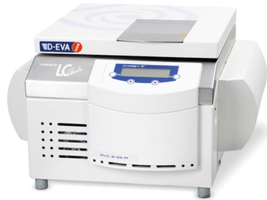
Figure 6: D-EVA Vacuum Centrifugation Evaporator used for Automated Evaporation of PFAS Extracts.
